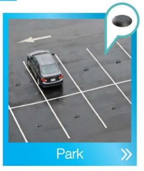
A battery operated floorbased sensor with a lifetime of 5 years identifies that the vehicle has arrived to the parking slot.
